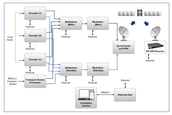
Figure 1.2 Typical Satellite Compression System
